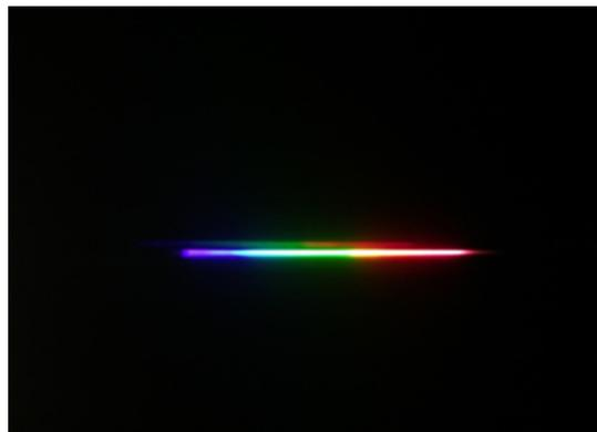
Figure 5-3: Spectra of a tungsten halogen lamp as imaged on the iPhone
