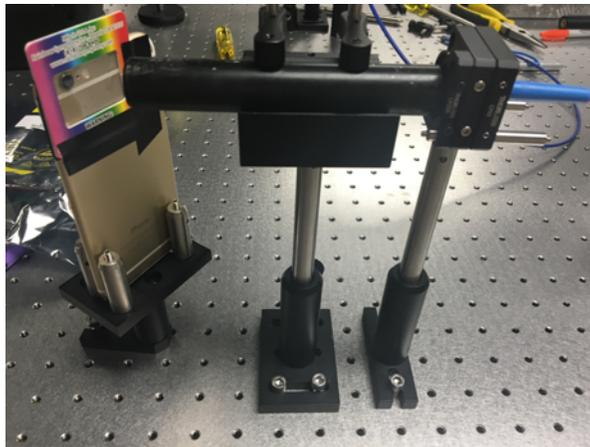
Figure 5-2: Bench top setup with a transmission grating
