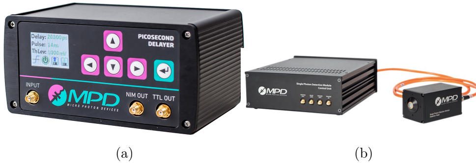
Figure 2.11: Figure 2.11a shows an image of the programmable delayer used in our system. Figure 2.11b shows the control unit coupled to the SPAD detection head with a wide-bandwidth cable
