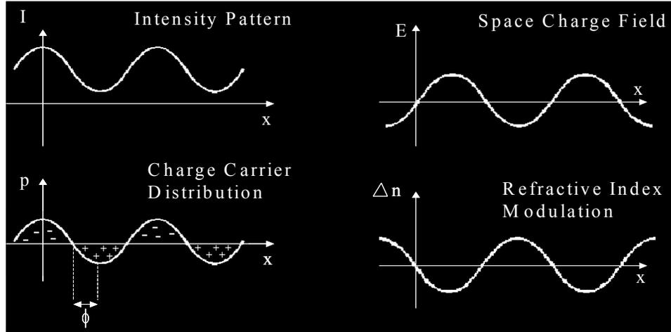
Figure 2, Photorefractive Effect
