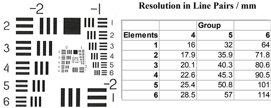
Figure 6, USAF Resolution Test Pattern
