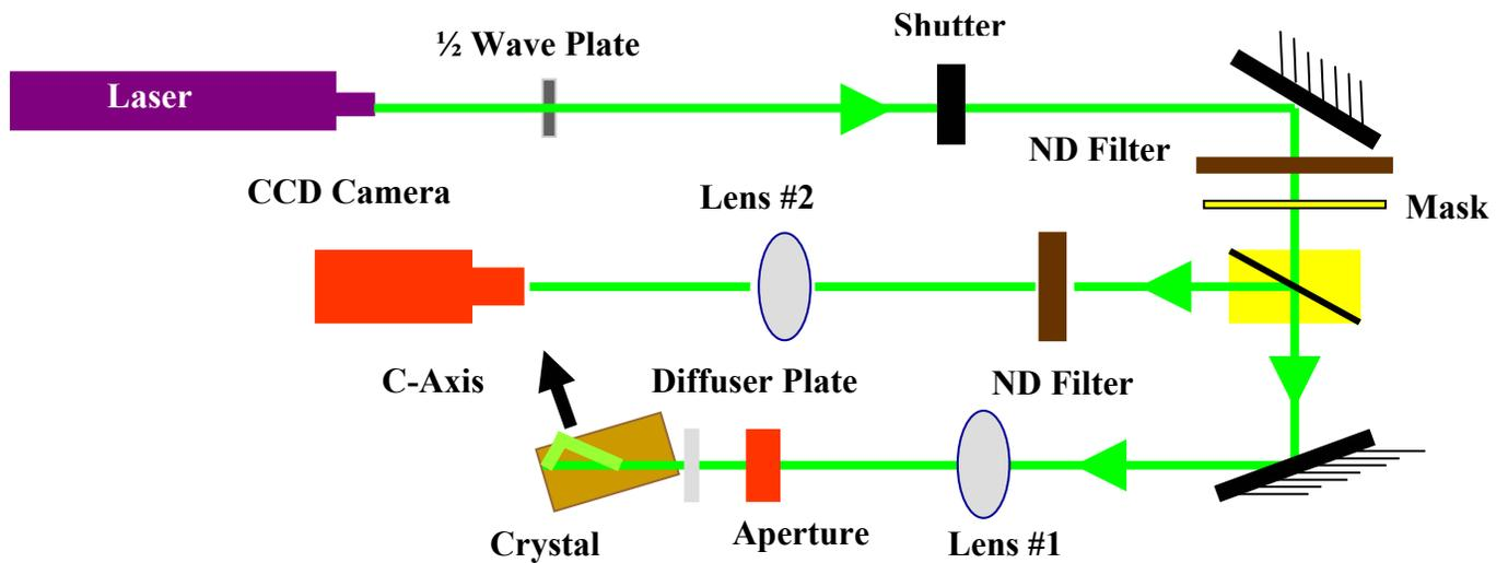
Figure 5 Experimental Set up of Phase Conjugation
