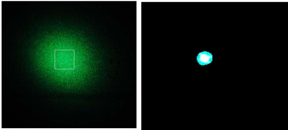
*Figure 7, Beam Through Diffuser Plate (left), Beam (right)*
