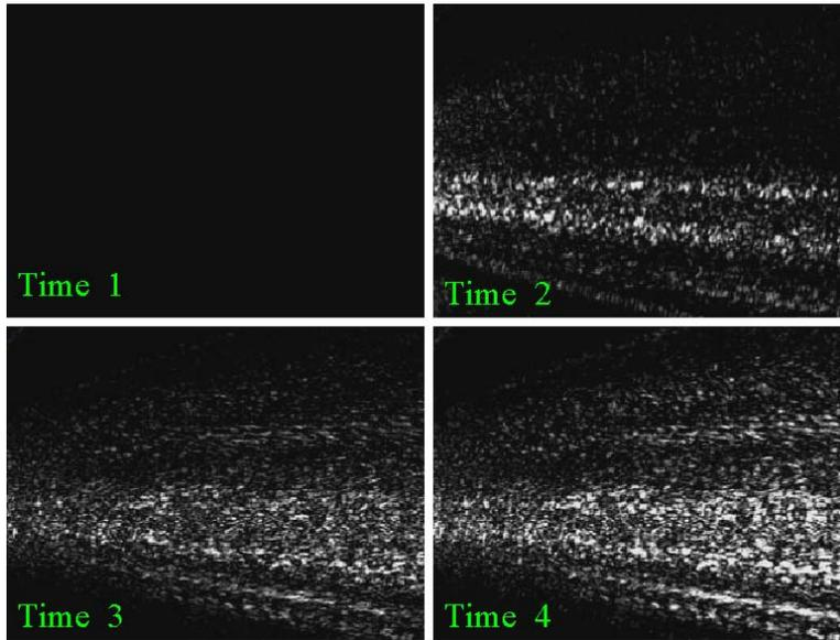
*Figure 8, a. Beam Fan Without Diffraction Grating*
