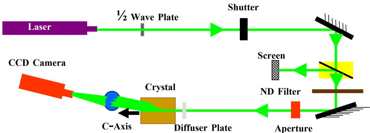
Figure 4 Experimental Set up of Beam Fanning
