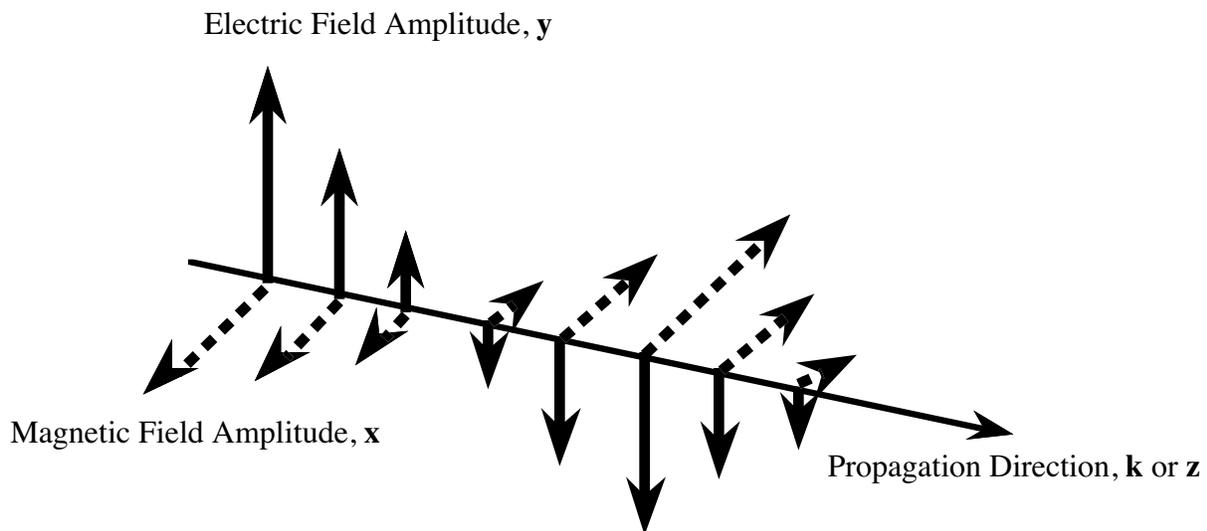
Figure 1: Linearly polarized light propagating in the  $z$  direction.
