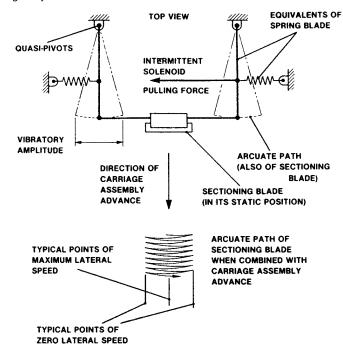
FIGURE 3. VIBRATOME 1500 SECTIONING SCHEMA
