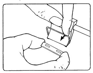
FIGURE 8 - SECTIONING BLADE MOUNTING
