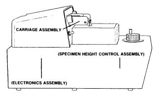
FIGURE 2. VIBRATOME 1500 FUNCTIONAL ASSEMBLIES
