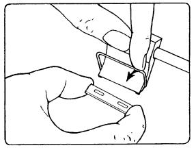
FIGURE 8 - SECTIONING BLADE MOUNTING
