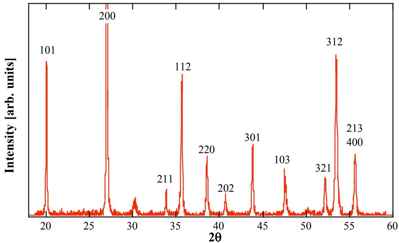
X-ray diffraction spectrum of zirconium silicate ( $\text{ZrSiO}_4$ ). The scattering angle  $2\theta$  is in degrees and the intensity is in arbitrary units. The diffraction peaks are labeled with the Miller index  $hkl$ . The unlabeled peak near  $30^\circ$  is due to a small amount of zirconium oxide ( $\text{ZrO}_2$ ).
