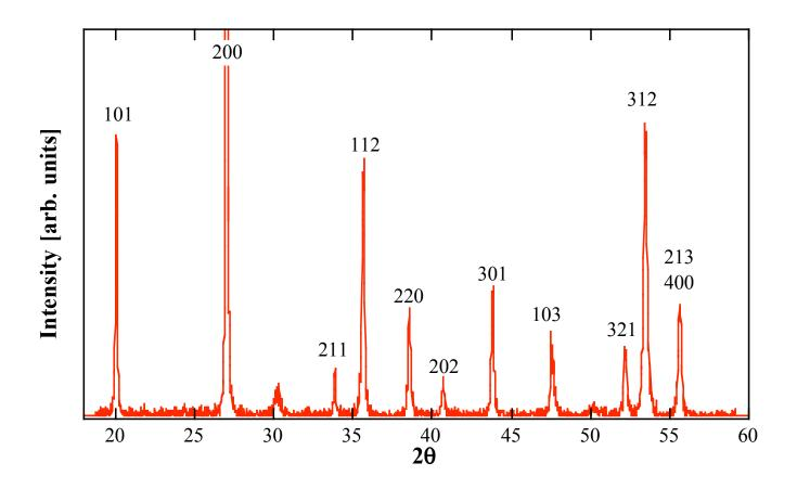
X-ray diffraction spectrum of zirconium silicate  $(ZrSiO_4)$ . The scattering angle 2 $\theta$  is in degrees and the intensity is in arbitrary units. The diffraction peaks are labeled with the Miller index *hkl*. The unlabled peak near 30° is due to a small amount of zirconium oxide  $(ZrO_2)$ .
