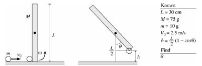
Solve: This is a two-part problem. Angular momentum is conserved in the collision, and energy is conserved as the ball rises like a pendulum. The angular momentum conservation equation about the rod's pivot point is
