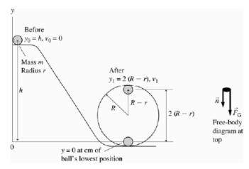
Solve: The marble's center of mass moves in a circle of radius R-r. The free-body diagram on the marble at its highest position shows that Newton's second law for the marble is
