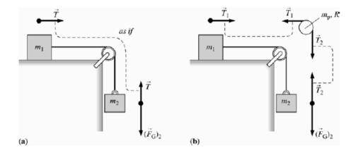
The free-body diagrams for the two blocks and the pulley are shown. The tension in the string exerts an upward force on the block  $m_2$ , but a downward force on the outer edge of the pulley. Similarly the string exerts a force on block  $m_1$  to the right, but a leftward force on the outer edge of the pulley.
