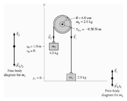
Because the pulley is not massless and frictionless, tension in the rope on both sides of the pulley is *not* the same. Solve: Applying Newton's second law to  $m_1, m_2$ , and the pulley yields the three equations:
