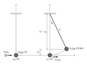
The figure shows three distinct moments of time: the time before the collision, the time after the collision but before the two balls move, and the time the 100 g ball reaches its highest point. We place the origin of our coordinate system on the 100 g ball when it is hanging motionless.
