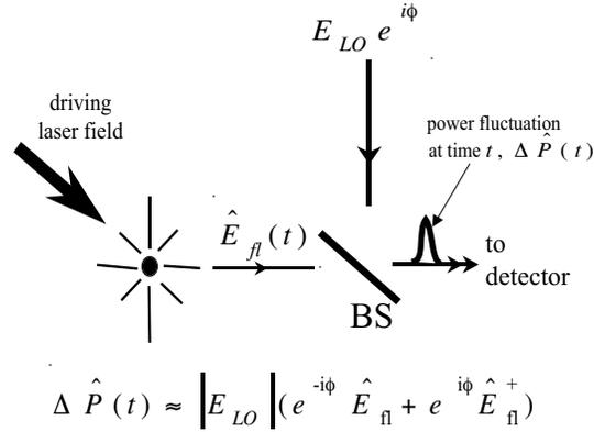
**Figure 1.** Measurement of phase-dependent effects in resonance fluorescence by homodyne detection. Fluorescence from a resonantly driven atom is mixed with a local oscillator field (LO) at a beamsplitter (BS). The LO is derived from the driving laser field.
