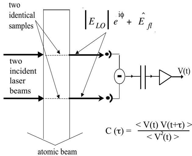
**Figure 2.** Outline of measurement of phase-dependent temporal correlations in resonance fluorescence by subtraction of transmitted power signals from two identically prepared atomic samples.
