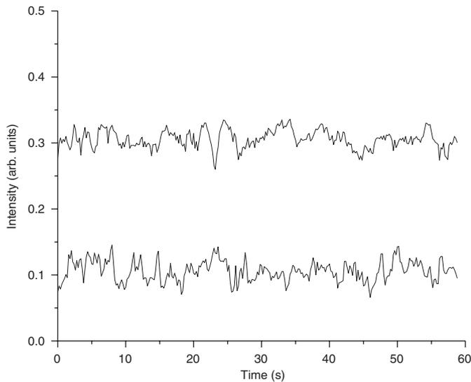
Fig. 2. The top plot shows a graph of intensity versus time for the center fringe in a Michelson interferometer with both arms located on the same optical table. The bottom plot shows the intensity versus time of the center fringe with the arms on different tables. The two plots are offset for clarity.
