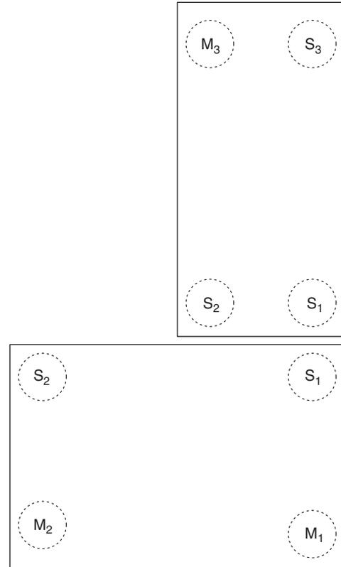
Fig. 1. Overhead view of the two table system highlighting the location of each “Master” (M) and its corresponding “Slaves” (S). M1 and M2 control slaves on both tables.
