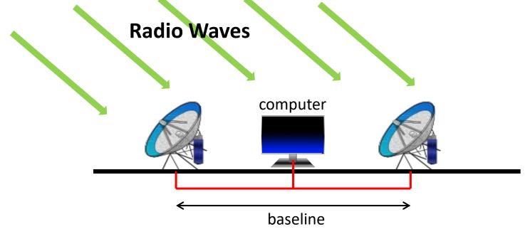
The computer combines the signals into an interference pattern; this allows the direction of the signal to be determined very accurately.
