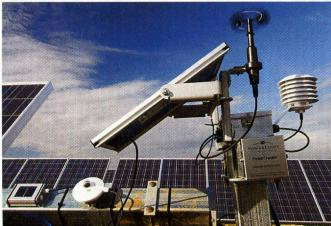
Serpa is about as sunny as central California. But even on a stormy day, the plant is productive. Sensor stations like the one above monitor the weather and the sun's location and control the angle of groups of solar panels. PowerLight's Wenger compares the rows of panels to slats on Venetian blinds: long, motorpowered metal beams attached
